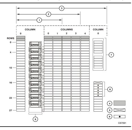
Figure 3-1. L180 Cartridge-Cell Arrays, CAP, and Drive Column (C67091)
