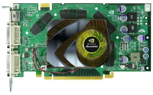
The NVIDIA® Quadro" FX 1500 graphics card provides Sun customers a mid-range 3D performance workstation graphics solution for professional MCAD applications. The Sun Ultra 40 M2 Workstation supports up to four NVIDIA Quadro FX 1500 graphics cards. This card ships with 256MB of DDR memory and can drive any two Sun displays, including two 24.1-inch LCD monitors.
