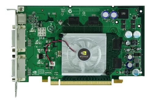
The NVIDIA® Quadro FX 560 graphics card provides Sun customers an entry-level 3D performance workstation graphics solution for SW development or everyday MCAD applications. This card ships with 128MB of DDR memory and can drive two Sun LCD displays .
