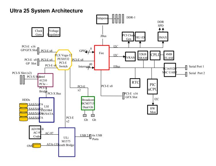
Figure 2. Sun Ultra 25 architecture block diagram
