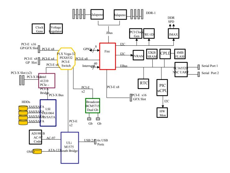
Figure 3. Sun Ultra 45 architecture block diagram
