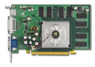
The NVIDIA® Quadro" FX 540 graphics accelerator provides Sun customers an entry-level 3D performance workstation graphics solution for SW development or everyday MCAD applications. This card ships with 128MB of DDR memory and can drive one Sun LCD display and one analog display. When the NVIDIA Quadro FX 540 a graphics card is installed, the ATI RageXL PCI graphics controller will be disabled.
