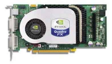
The NVIDIA® Quadro" FX 3450 graphics accelerator provides Sun customers a high-end 3D performance workstation graphics solution for professional MCAD. This card ships with 256MB of DDR memory and can drive any two Sun displays, including two 24.1-inch LCD monitors. When the NVIDIA Quadro FX 3450 a graphics card is installed, the ATI RageXL PCI graphics controller will be disabled.
