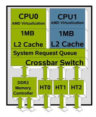
Figure 4 – Block Diagram of the AMD Opteron 1200-series Processor
