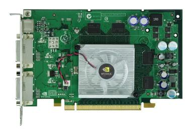
Figure 13 – Connector of the NVIDIA Quadro FX 560 Graphics Accelerator Card
