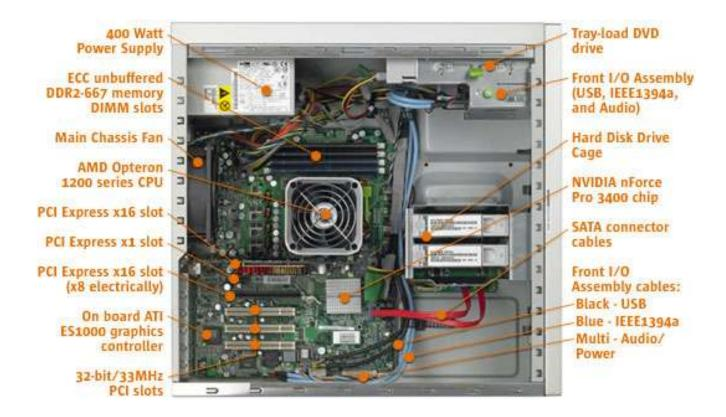
Figure 2 – Internal View of the Sun Ultra 20 M2 Workstation
