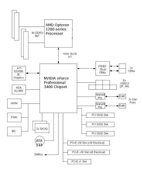
Figure 3 – Block Diagram of the Sun Ultra 20 M2 Workstation
