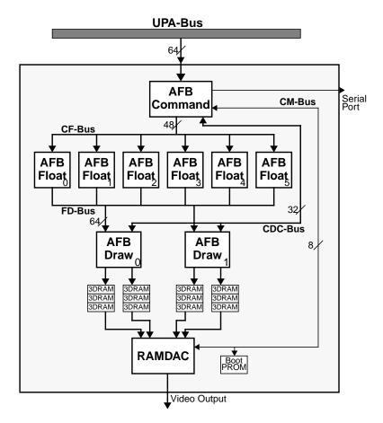
Figure 3. Sun Elite3D chip-level diagram
