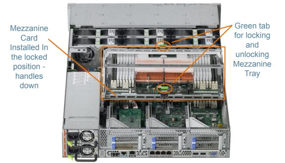
Figure 21. Sun Fire X4440 with Mezzanine Board Installed
