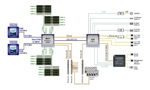
Figure 4. Sun Fire X4150 SAS Server Block Diagram
