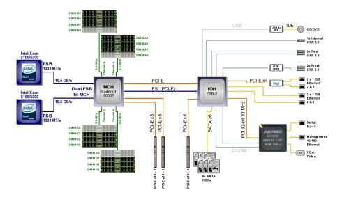
Figure 3. Sun Fire X4150 SATA Server Block Diagram
