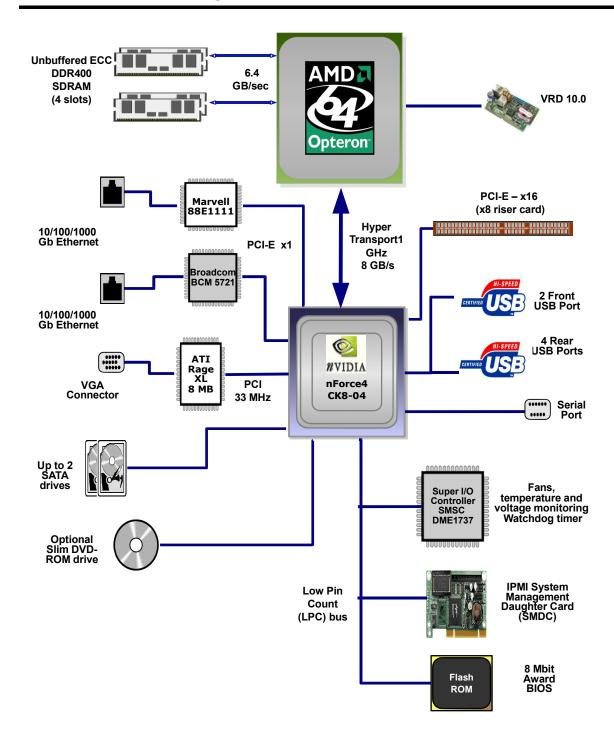
Figure 3.Sun Fire X2100 Server System Architecture
