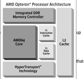
Figure 1. Architecture block diagram for the AMD Opteron processor
