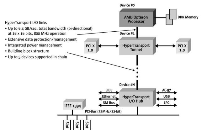
Figure 2. Sample HyperTransport technology interconnect block diagram
