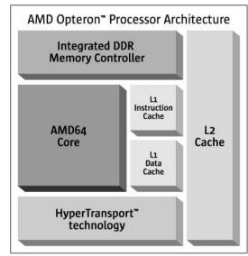
Figure 1. Architecture block diagram for the AMD Opteron
