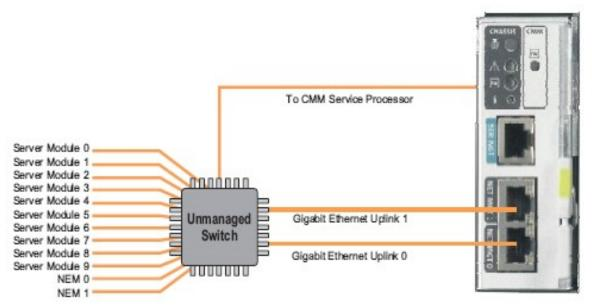
The functions of the X6440 Service Processor is independent of the operating system, so that the same level of manageability is provided regardless of the choice of OS. The SP is available for Server Module management even when the Server Module is powered off, but the chassis is powered on.
