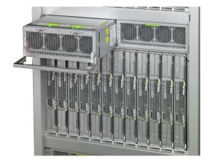
Power Supply Module Removed
