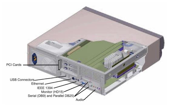
Figure 3. Rear view of Sun Blade 150 workstation, showing connectors
