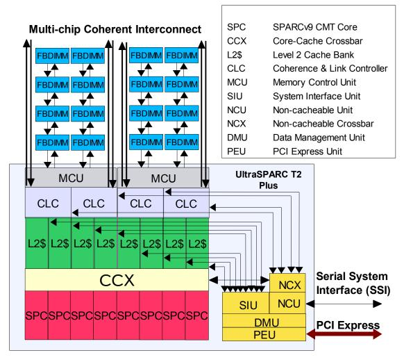
Figure 2 - UltraSPARC T2 Plus Block Diagram
