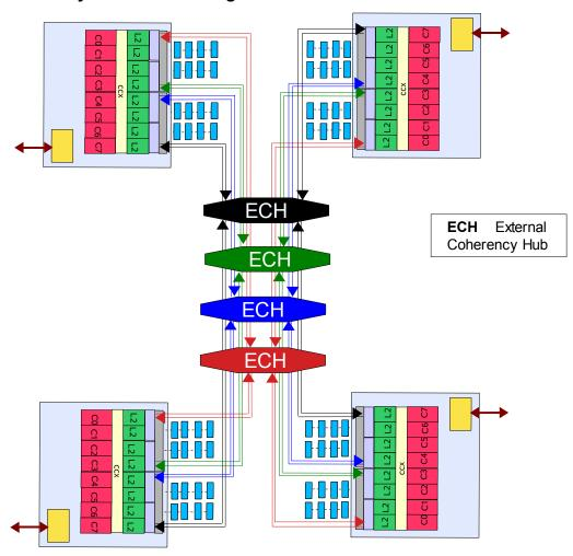
Figure 3 - External Coherency Link
