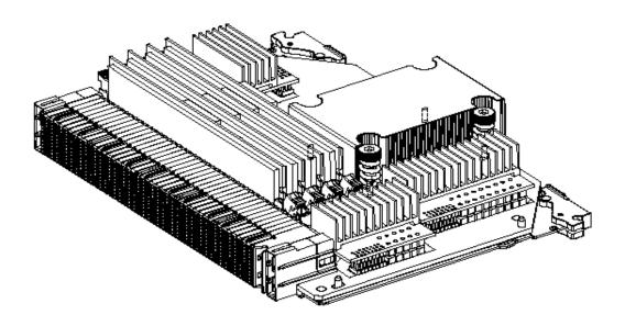
Figure 5 - CPU Board 3-D View and FB-DIMM Location
