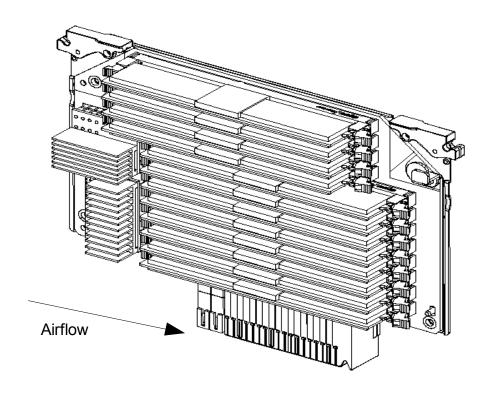
Figure 6 - Memory Board 3-D View and FB-DIMM Location
