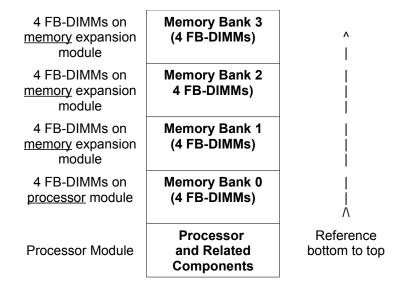
Figure 13 – Logical Representation of One Processor and Associated Memory Expansion Module
