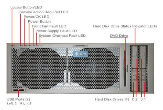
Figure 10 - System Cabinet, Front View
