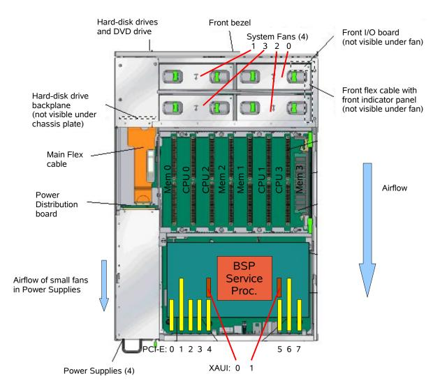
Figure 12 - System Cabinet, Top View
