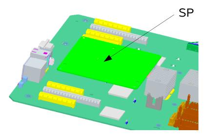
Figure 7 – Service Processor Module
