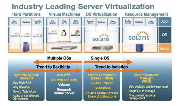
Figure 9 - Virtualization Structure
