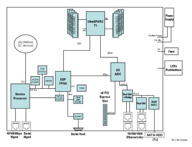
Figure 4. Sun SPARC Enterprise™ T1000 server block diagram
