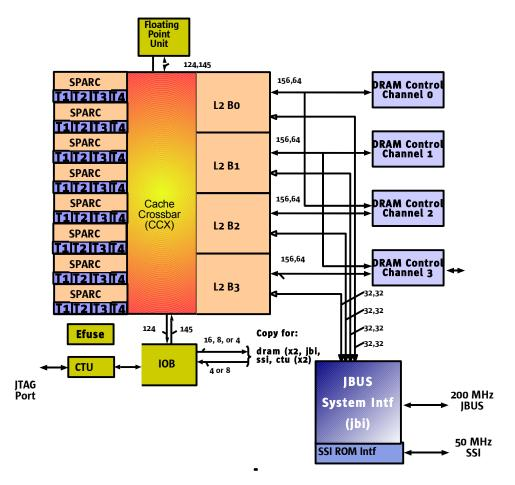
Figure 2. The UltraSPARC T1 multicore processor block diagram (Note: Sun SPARC Enterprise T1000 server utilizes two memory controllers)
