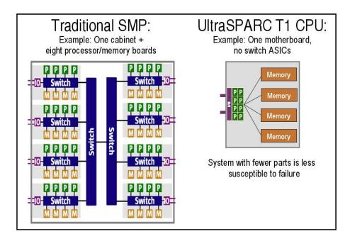
Figure 3. Traditional SMP vs. UltraSPARC T1 CPU design
