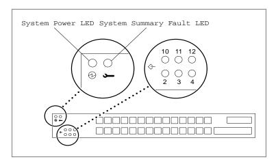
Figure 3. Front Panel System Power/Fault Indicators
