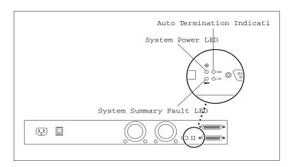
Figure 7. Rear Panel LEDs
