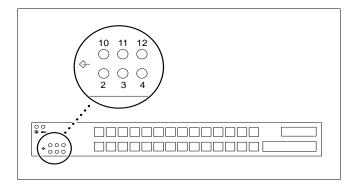
Figure 4. Front Panel Disk Drive LEDs
