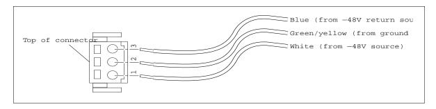
Figure 9. DC input power cables
