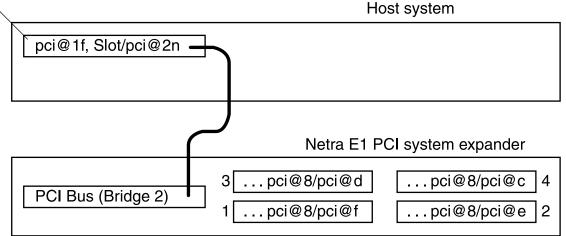
Figure 7. Logical and Physical Device Numbers With One System Expander
