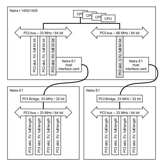
Figure 10. Netra 1400 Server or Netra 1405 Server Connected to Two Netra E1 PCI System Expanders
