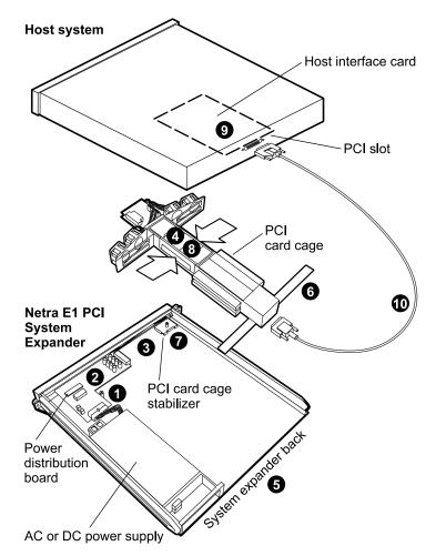
Figure 6. Netra E1 PCI System Expander Installation
