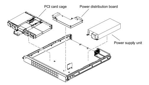
Figure 3. Netra E1 PCI System Expander Internal Components. The components are accessible by removing one screw from the top cover.
