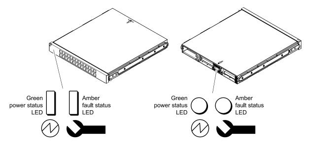
Figure 2. System Icons, Power, and Fault LEDs
