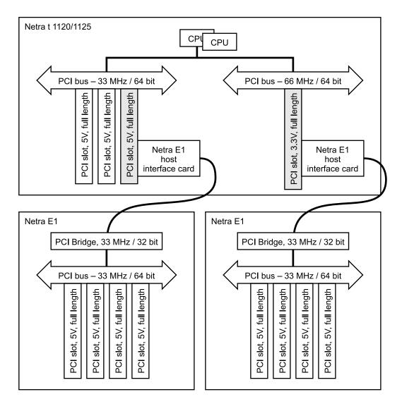
Figure 9. Netra 1120 Server or Netra 1125 Server Connected to Two Netra E1 PCI System Expanders
