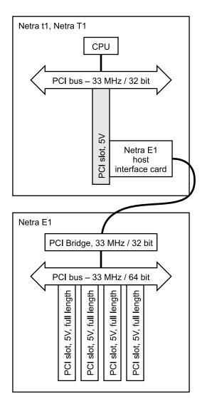
Figure 8. Netra t1 or Netra T1 Server Connected to a Netra E1 PCI System Expander
