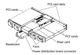
Figure 4. Netra E1 PCI System Expander PCI Card Cage
