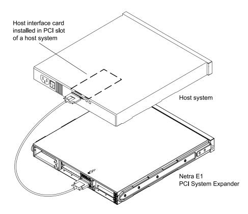
Figure 1. Netra E1 PCI System Expander Cabled to the Host Interface Card
