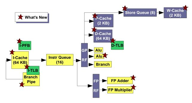
Figure 4: UltraSPARC IV+ enhancements (enhanced components are starred)
