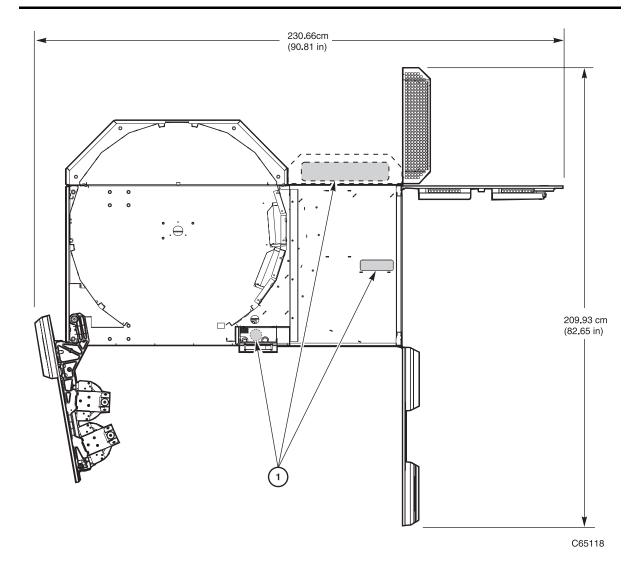
Figure B-2. Top View of Library Showing Cable Access
