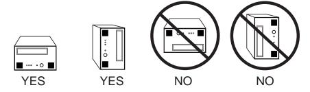
Figure 4. Acceptable mounting orientations for the internal Viper 200
