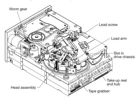
Figure 13. Diagram of Viper 200 showing key components used in manual cartridge removal (no tape cartridge in drive)
