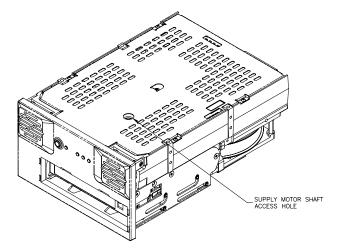
Figure 15. Diagram of underside of Viper 200 showing supply motor access hole
