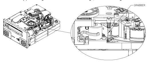
Figure 16. Diagram of underside of Viper 200 showing tape grabber near cartridge
