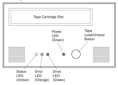
Figure 9. Generic front panel display for Viper 200
