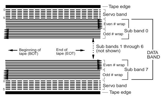
Figure 18. Layout of tracks on LTO Ultrium tape
