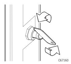
• If you are replacing the operator panel or rack installed components: Open the rack door by pulling gently on the left side of the door.
