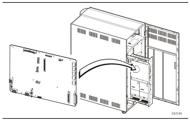
**Note:** Depending on your library's configuration, you might need to remove MPV card assembly (CPCI module) from the old MPC card and install it onto the new MPC card.
