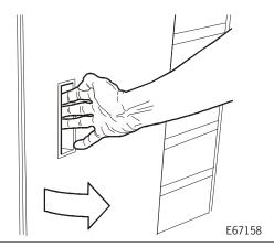
3. Remove power from the library by pressing down on the power switch on the bottom left area of the library.
