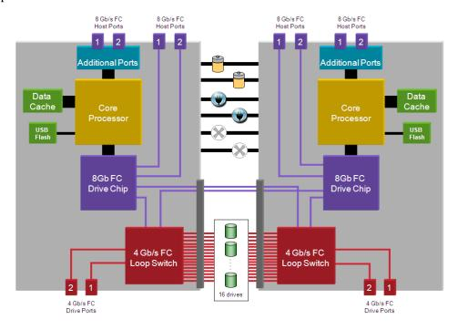
Figure 3. Sun Storage 6180 — 4GB Cache -8 Host Port FC RAID Controller Card
