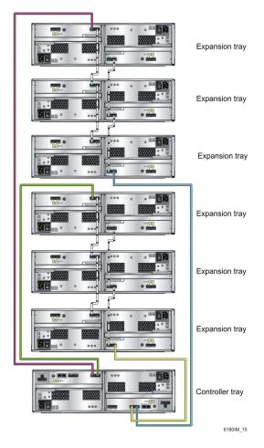
Figure 9. Sun Storage 6180 and CSM200 Cabling
