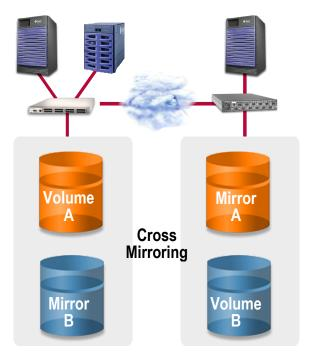
Figure 13. Sun StorageTek Data Replicator Software
