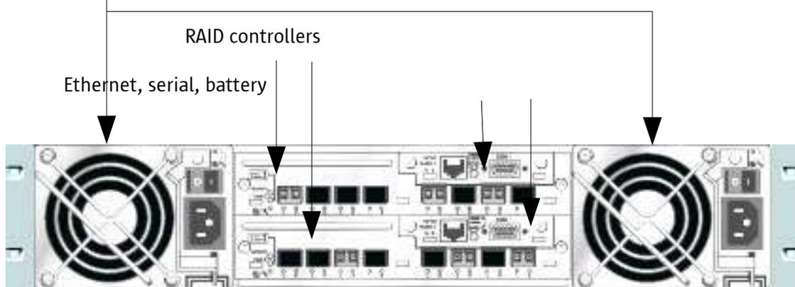
Figure 2. Major components, RAID array
