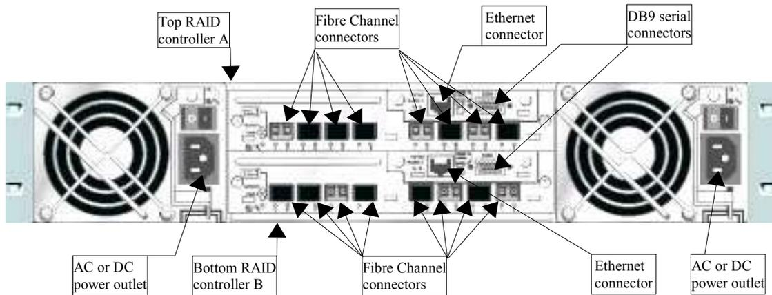
Figure 3. Rear panel of RAID array, dual controller configuration
