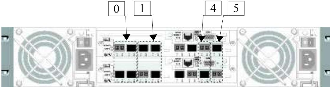
Figure 10. Four discrete loop segments (host port channels 0, 1, 4, 5)
