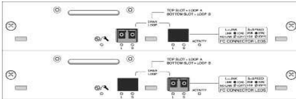
Figure 6. RAID-I/O FRU, Sun StorEdge 3511 Fibre Channel array (single RAID controller configuration)
