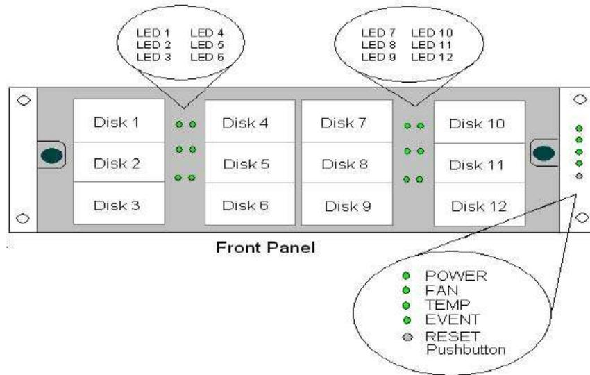
Figure 16. Front panel of the Sun StorEdge 3511 Fibre Channel array
