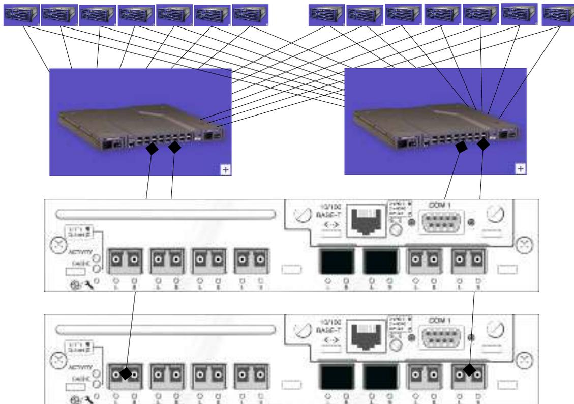
Figure 15. Four 2-Gb Fibre Channel point to point connections, full fabric, two 16-port switches, 14 hosts
