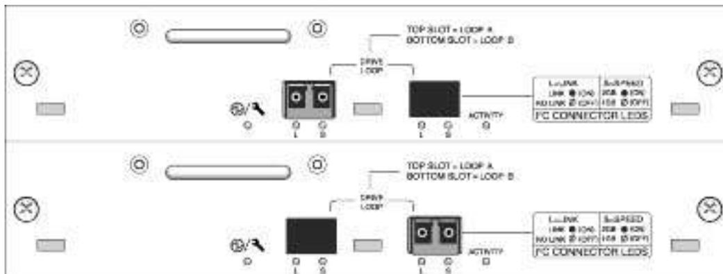
Figure 8. Expansion-I/O modules, Sun StorEdge 3511 Fibre Channel array
