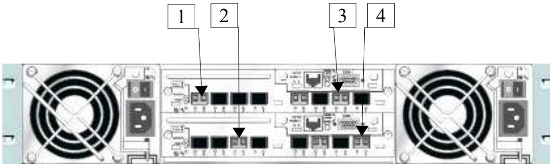
Figure 14. Four 2-Gb Fibre Channel point to point connections
