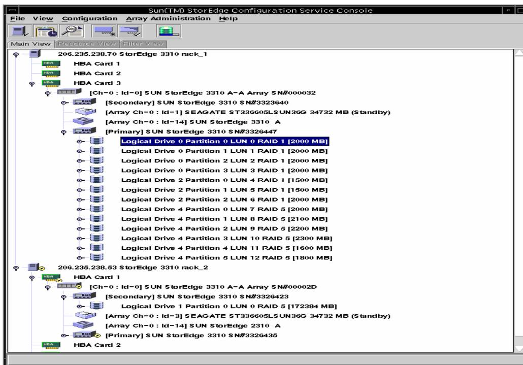
Figure 19. Sun StorEdge Configuration Service GUI
