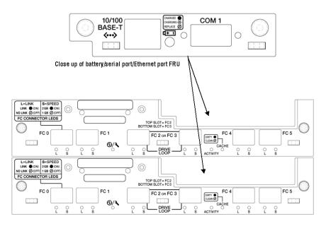
Figure 5. RAID-I/O FRU, Sun StorEdge 3510 Fibre Channel array (dual RAID controller configuration)
