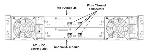
Figure 7. Rear panel of expansion array Storage Expansion Fibre Channel I/O Ports
